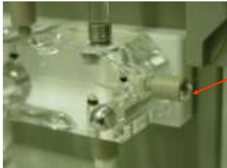
Urea crystals have formed due to a small leak where the capillary comes into the pump block
