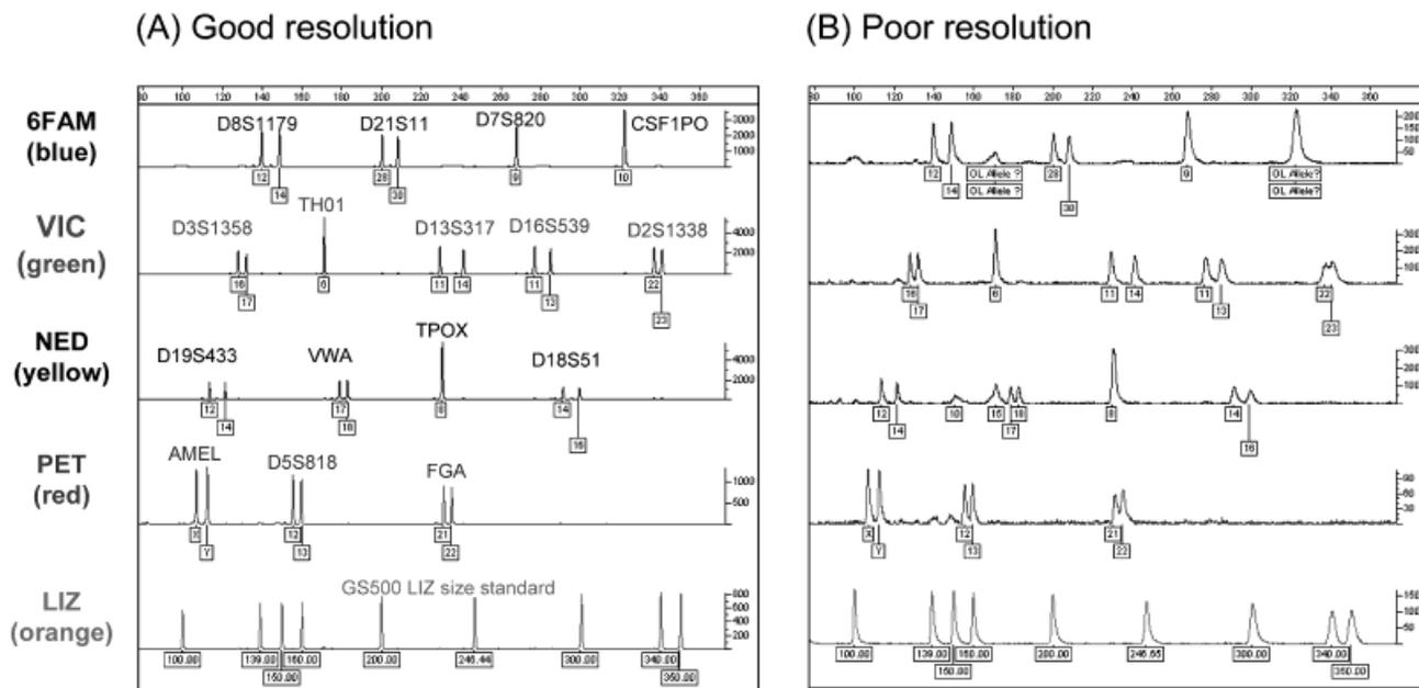
**Figure 6.** Comparison of same sample with (A) good resolution and (B) poor resolution due to a bad capillary. The STR kit used was the AmpFISTR® Identifier™ (5-dyes).
