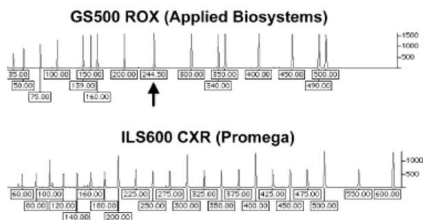
**Figure 5.** Two different internal size standards commonly used with STR typing. The ~245 bp peak (arrow) in the GS500 ROX standard is not included in the software calculations.
