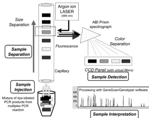
**Figure 2.** Schematic illustration of the separation and detection of STR alleles with an ABI Prism 310 Genetic Analyzer.
