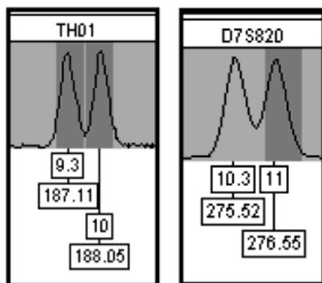
**Figure 8.** Resolution of STR variant alleles containing single-nucleotide spacing on ABI 3100 with POP-6 polymer. These TH01 alleles 9.3/10 and D7S820 alleles 10.3/11 were observed when typing samples in a previous study [70].
