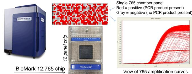
Utilizes a microfluidic chip to partition the PCR mastermix into 765 chambers (volume of each chamber = 6 nL).
