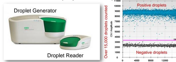
The QX100 droplet generator partitions samples containing DNA template into 20,000 nanoliter-sized droplets. After PCR in a standard thermal cycler (9700, Veriti, etc), the droplets from each sample are streamed in single file through the QX100 droplet reader. The PCR-positive and PCR-negative droplets are counted to provide absolute quantification of target DNA in digital form.
