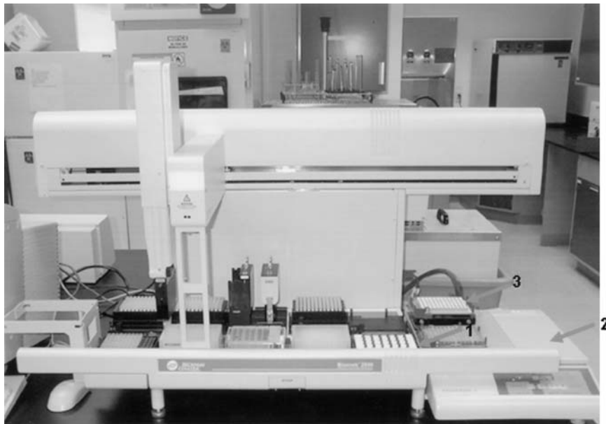
FIG. 1—BioMek® 2000 robot with modifications for the application of the DNA IQ™ System for DNA extraction. Numbers and arrows refer to specific additions. 1 = magnet (Magnabot), 2 = shaking platform, 3 = thermal exchange unit.
