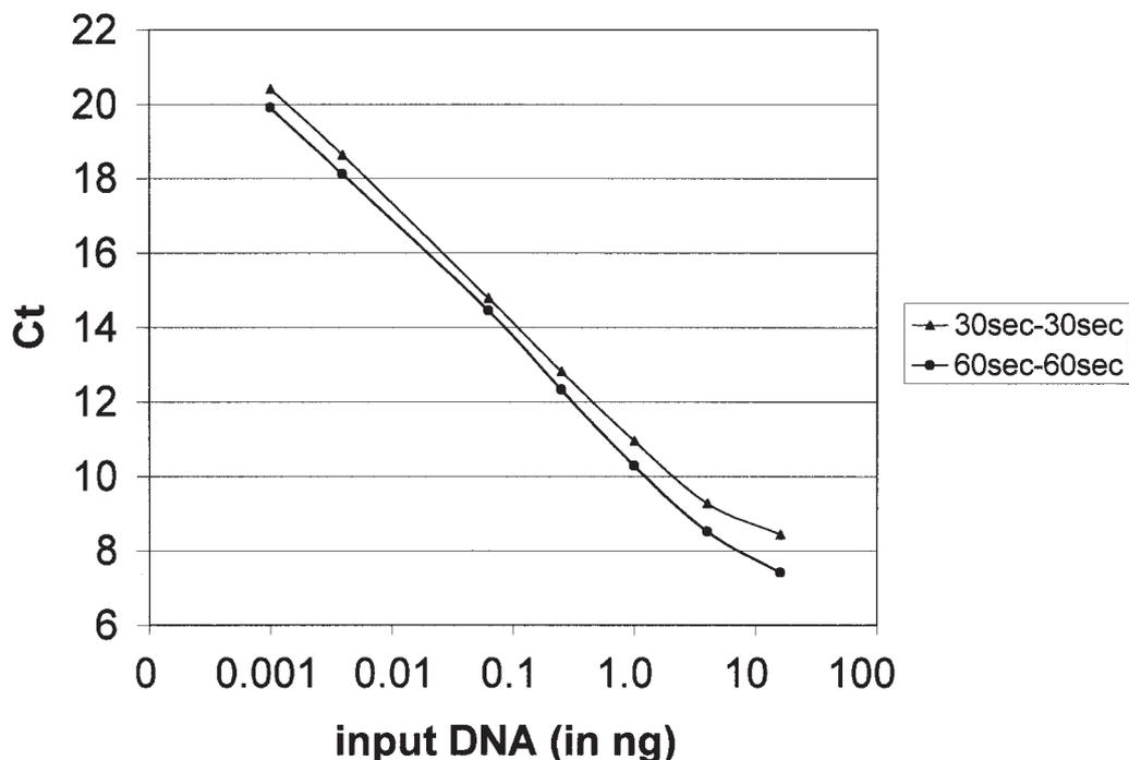
FIG. 3—Plot of the  $C_t$  values versus input human DNA standard for 60-s anneal/60-s extension (black circles) versus 30-s anneal/30-s extension (gray triangles). The curves are of identical shape with the  $C_t$ s, just slightly higher for the 30-s anneal and 30-s extension.
